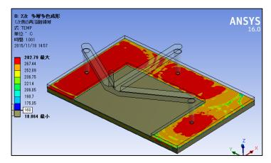
Figure 1: Temperature profile of the re-melted areas (160  $^{\circ}\!\!C$  or more) of the product of the first molding
