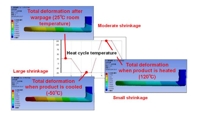
Figure 3: Profiles of the total amount of deformation of a product in a heat cycle test based on a temperature of 25°C at the time of warpage.
