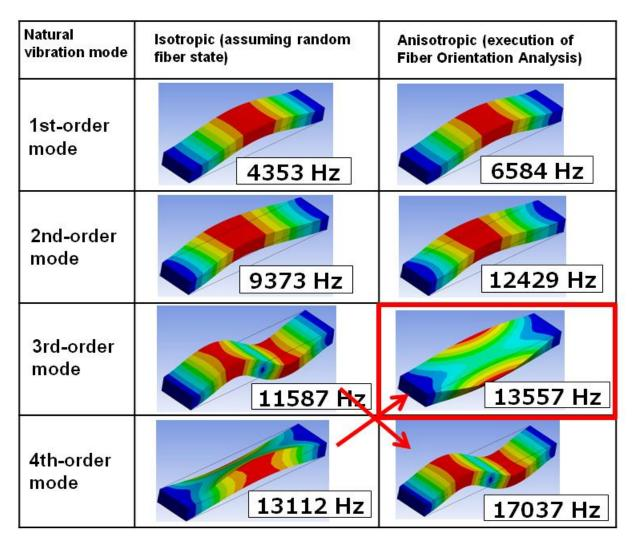
Figure 2: Natural frequency analysis results (natural vibration modes up to the 4th order) for a plate-shaped composite material fixed at both ends. The left side is an isotropic material (random fiber state) and the right side is an anisotropic material (execution of PlanetsX Fiber Orientation Analysis). In the deformation of the anisotropic material, the third-order and fourth-order modes have swapped places compared to the isotropic material.
